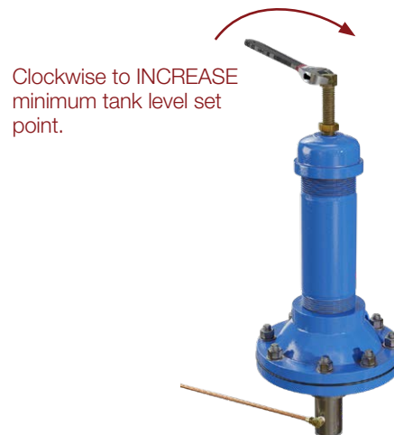
Figure 3 Model 27 - Altitude Pilot
