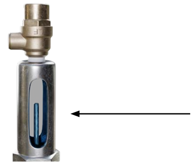
Figure 5 Position Indicator Stem in UP Position Indicating Valve OPEN
