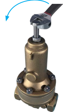
Figure 4 PV20C — Pressure Sustaining Control
