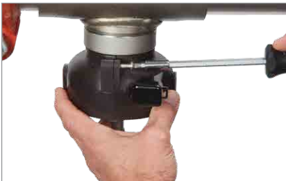
3. Insert the bolts and tighten.
