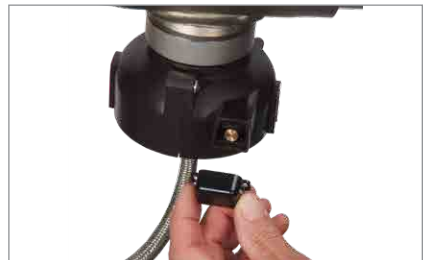
4. Remove the dust cover from the sensor.
