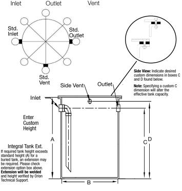
Verify all selections with your local Orion rep - tank products and accessory equipment are non-cancelable & non-returnable. **Note:** Tanks are made to +0.25 in. tolerance.
