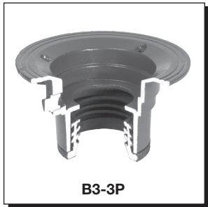
B3 Body, 3" Push-on connection standard with trap primer tapping.
