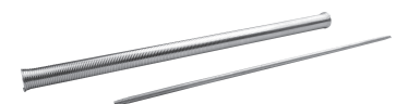
Spring benders are used with RadiantPEX-AL tubing to prevent over bending and kinking of the tubing. Spring benders are not needed for RadiantPEX+ or RadiantPERT.
