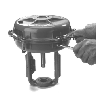
Fig 1 - Remove Housing Bolts
