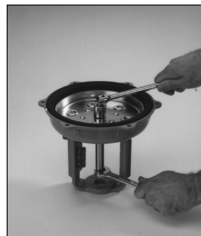
Fig 2B - Remove Springs, Stem Nut
