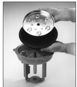
Fig 2C - Remove Washers, Thrust Plate, Diaphragm
