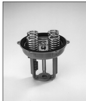
Fig 5 - Reverse Replacement of Diaphragm and Thrust Plate. Four (4) springs shown. See note on page 5.
