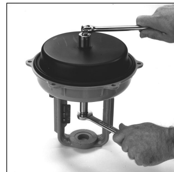
Fig 2B - Remove Stem Nut, & Washers
