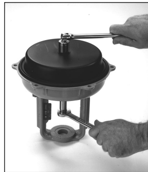
Fig 2A - Remove Upper Housing, Stem, Nut and Washers
