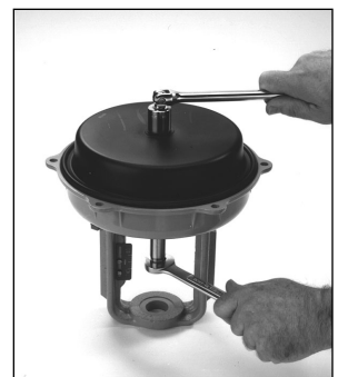
Fig 6 - Replace Washers, Tighten Stem Nut
