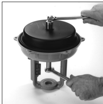
Fig 2 - Remove Stem Nut, and Washers
