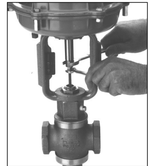
Fig 3 - Loosen Stem Locknuts
