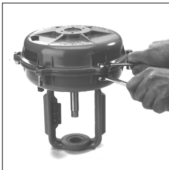
Fig 1 - Remove Housing Bolts
