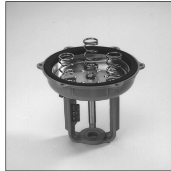
Fig 2 - Remove Upper Housing
