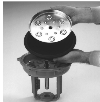
Fig 4 - Remove Thrust Plate and Old Diaphragm
