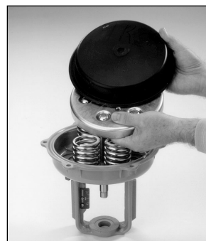
Fig 5 - Replace Springs, Reversed Thrust Plate and Diaphragm
