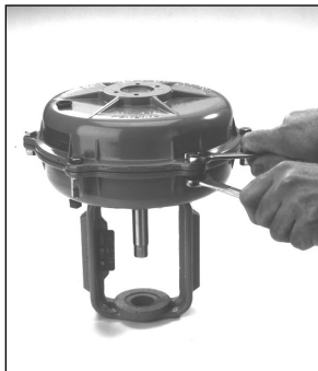
Fig 1 - Remove Housing Bolts
