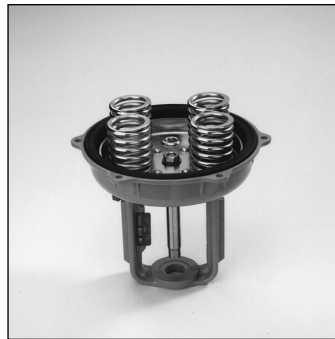
Fig 2 - Remove Upper Housing, Remove Springs (4 Shown)
