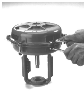
Fig 1 - Remove Housing Bolts
