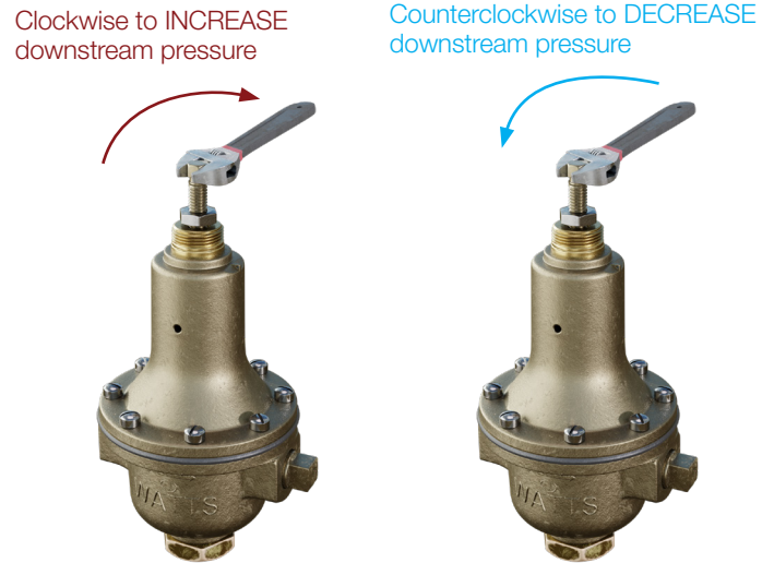
Figure 2 CP15 — Pressure Reducing Control
