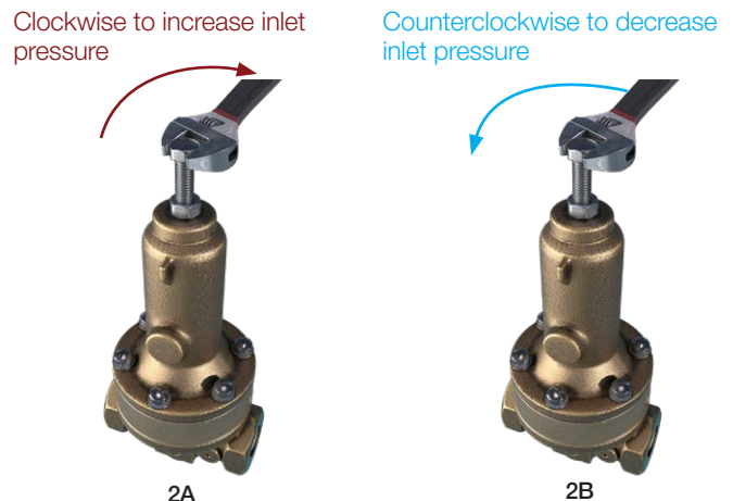
Figure 2 PV20C — Pressure Sustaining Control
