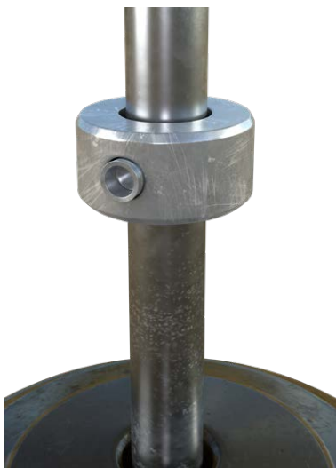
Close-up of Stop-Collar
