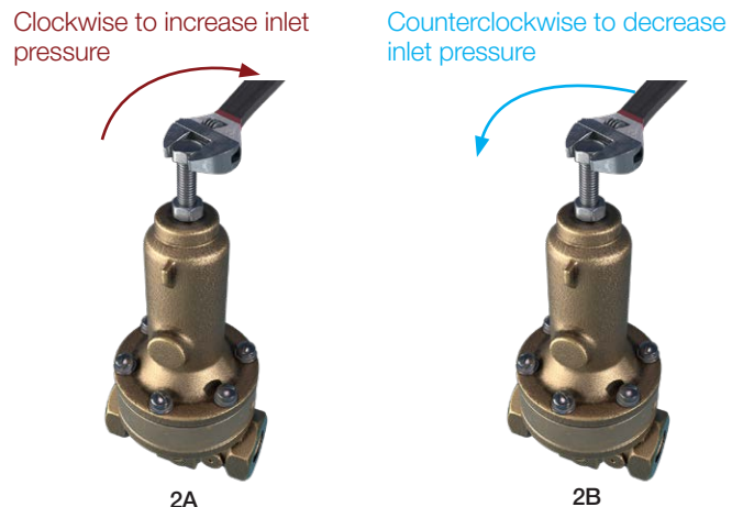
Figure 2 PV20C — Pressure Sustaining Control
